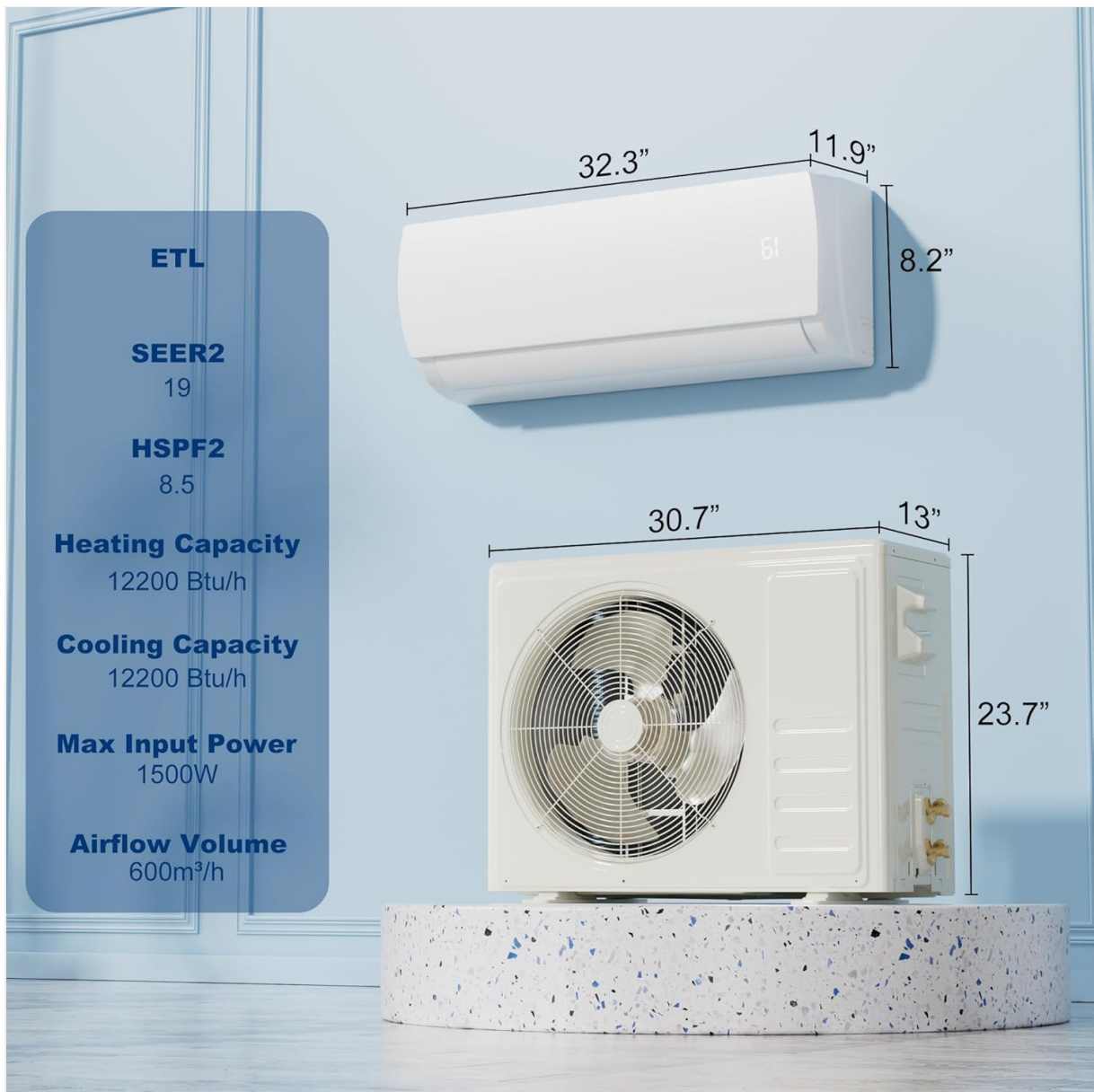
Image: A diagram illustrating the dimensions of both the indoor and outdoor units of the Uthfy HY12GWH115 Split Air Conditioner, along with key performance metrics such as SEER2, HSPF2, heating/cooling capacity, max input power, and airflow volume.
