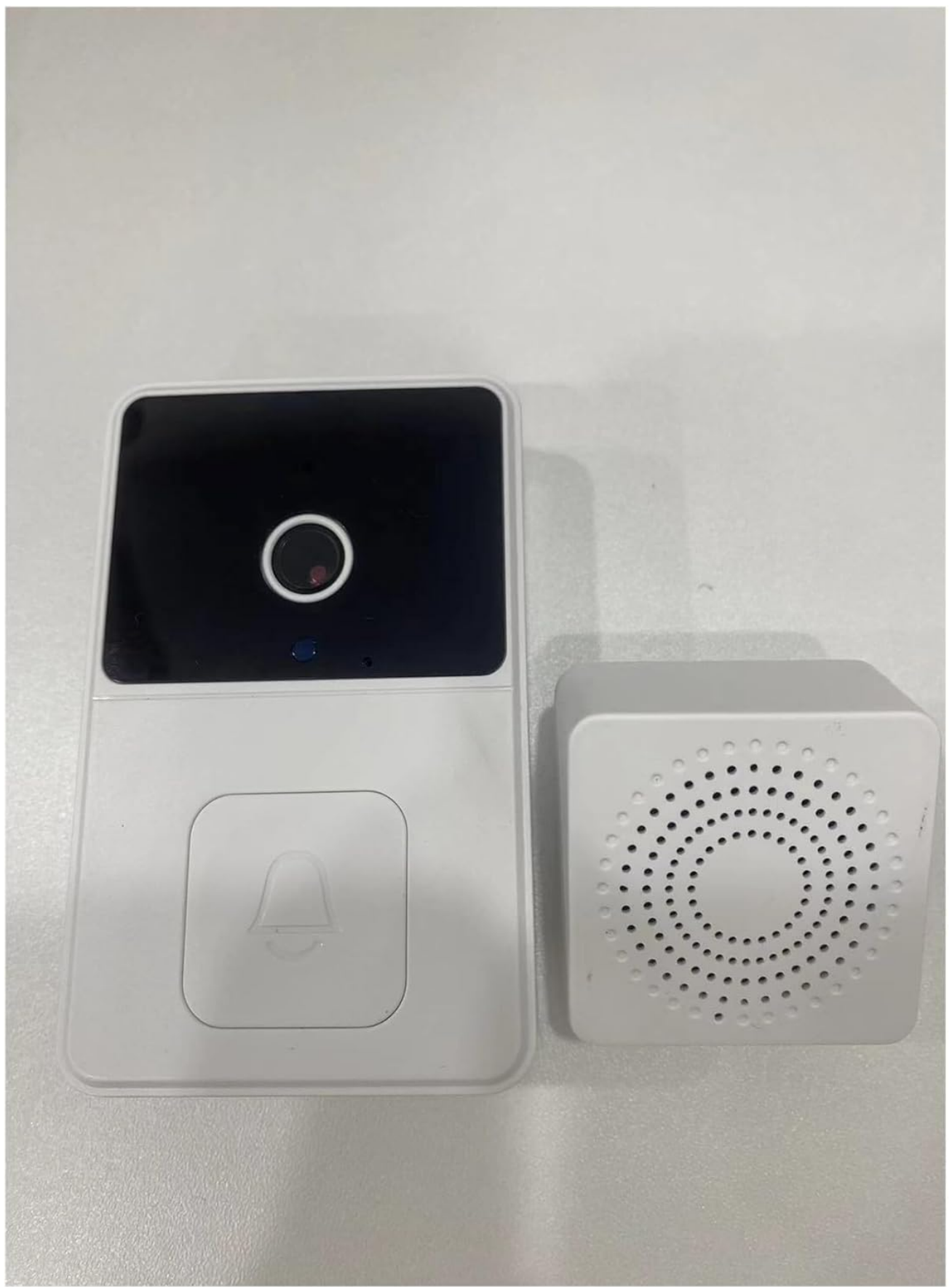
Figure 1.1: The M8 Wireless Doorbell Camera (left) and its accompanying Chime unit (right).
