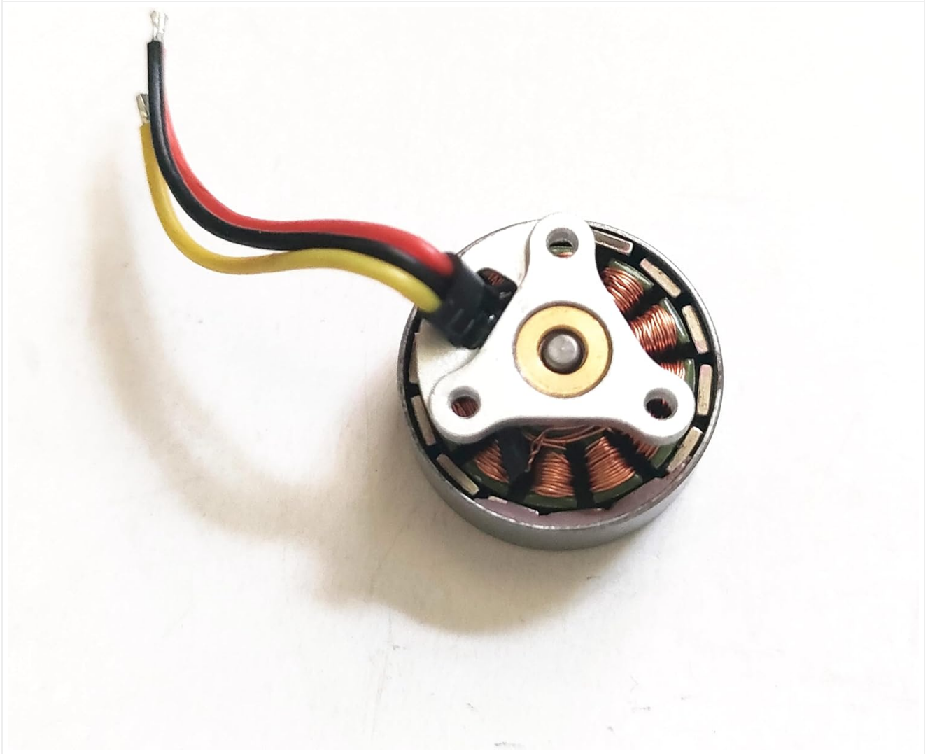
Figure 3.1: Bottom view of a single brushless motor, showing the three connection wires (red, yellow, black) and mounting holes.
