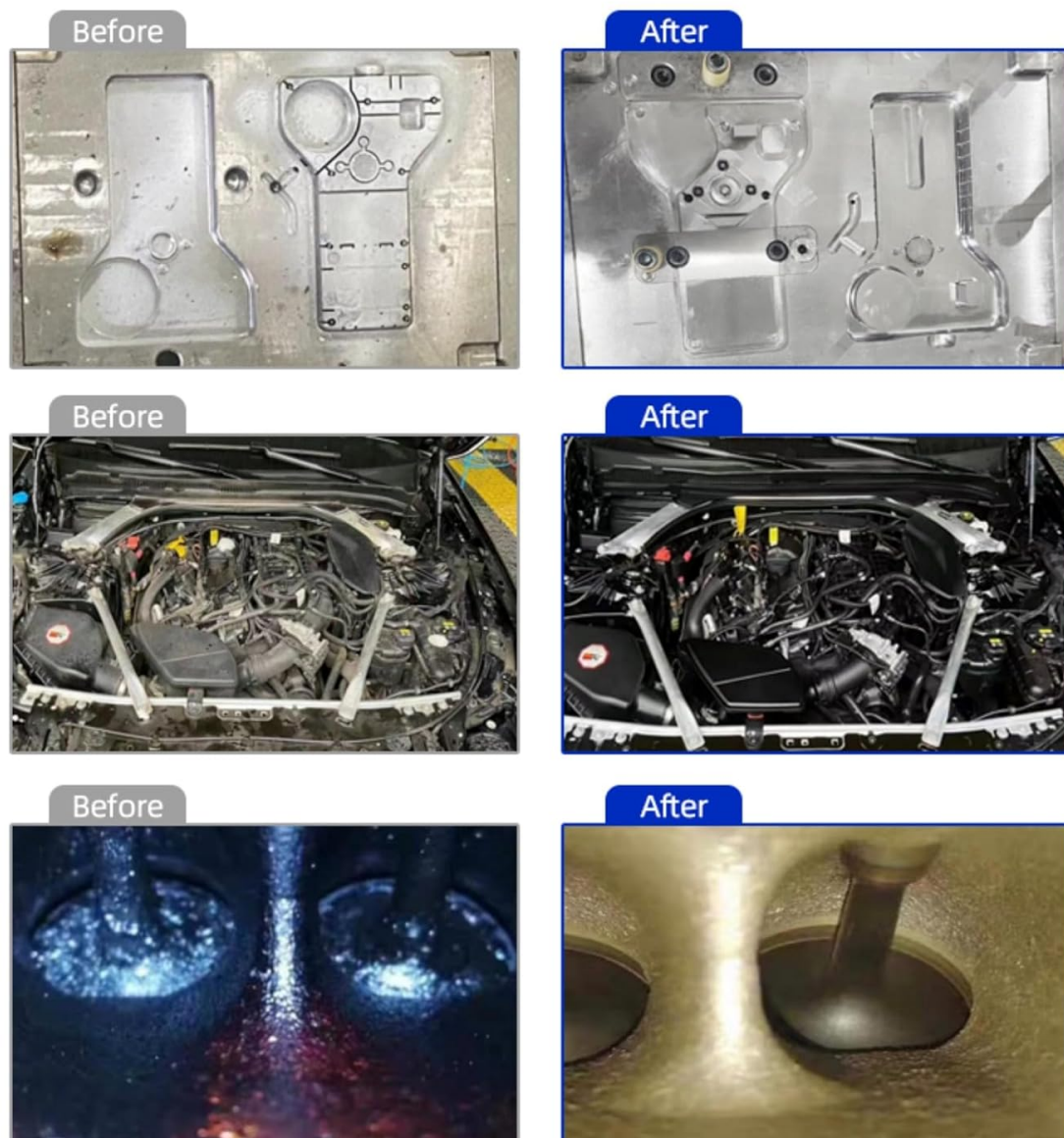
Figure 5.1: Examples of cleaning effectiveness on various surfaces, including industrial molds, engine components, and valves.
