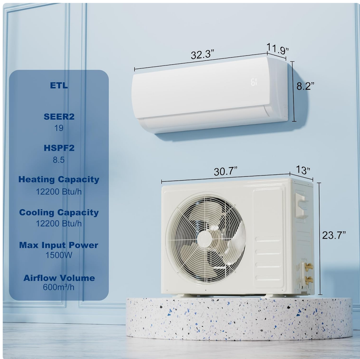
Image 7.1: Dimensions and key performance specifications of the Uthfy HY12GWH230.
