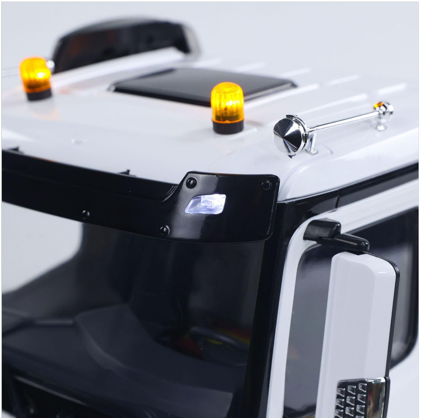
Image: Close-up view of the cab's roof-mounted warning lights and front auxiliary lights.
