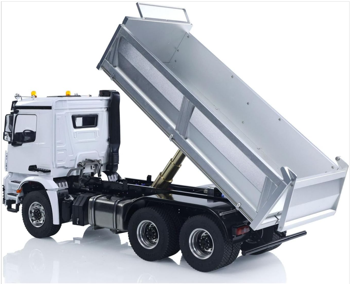
Image: Rear-side view of the dumper truck with its bed fully raised, demonstrating the hydraulic lifting capability.
