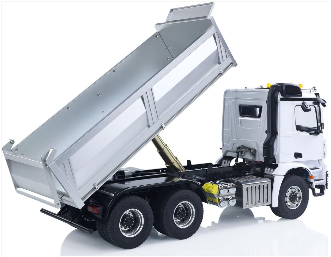
Image: Side view of the dumper truck with its bed fully raised, showing the extent of the hydraulic lift.
