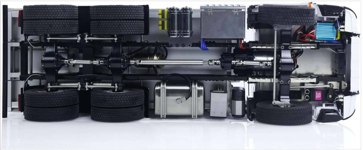
Image: Underside view of the truck chassis, revealing the detailed metal axles, drivetrain, and suspension components.
