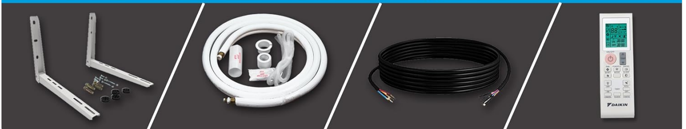
Figure 2: Detailed view of the Maxwell all-inclusive installation kit. Items include 15' Gas & Liquid Insulated Copper Lines, Stranded and Unshielded 16 Gauge 4 Lead Interconnecting Cable, Wall Filler Putty, Decorative Wall Cap, Wall Sleeve Cylinder, Outdoor Unit Wall Bracket, Non-Adhesive Decorative Wrapping Tape, and 6 Ft. Long Flexible Condensate Drain Hose.
