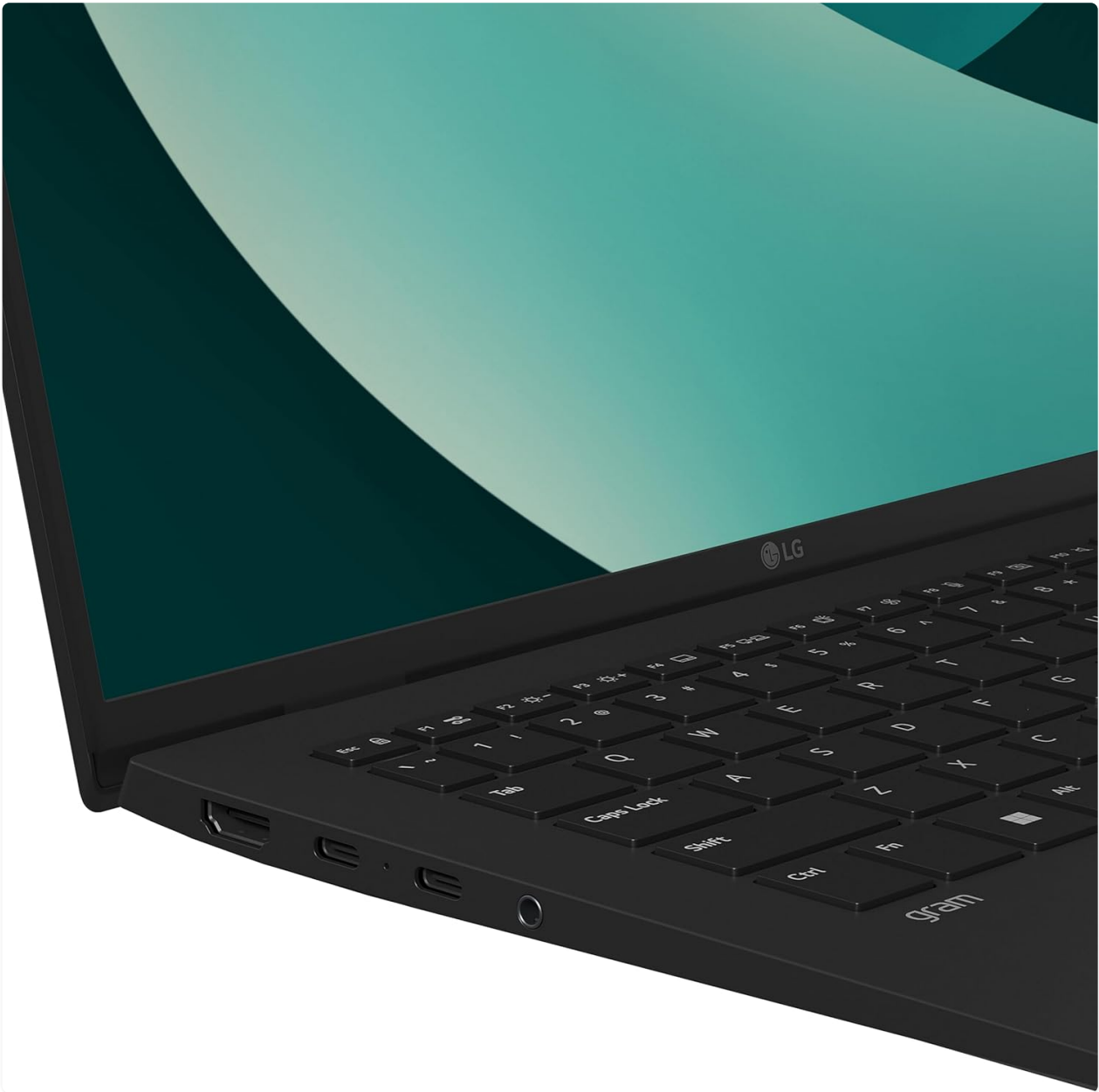
Figure 4: Left side ports (Thunderbolt 4, HDMI, Headphone/Mic).
