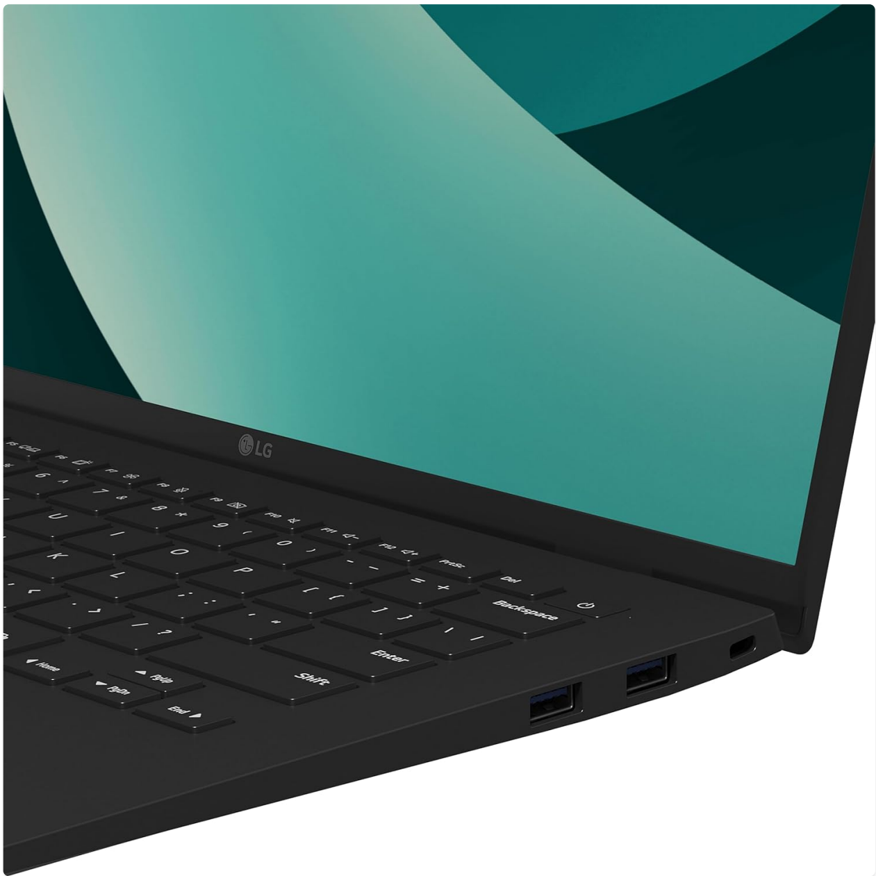
Figure 5: Right side ports (USB 3.2 Gen2).
