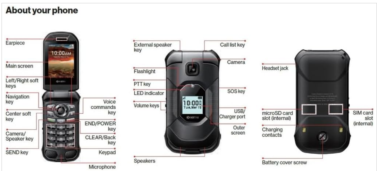
Figure 2.1: Key components of the KYOCERA DuraXA Equip E4831, including internal and external features, and port locations.
