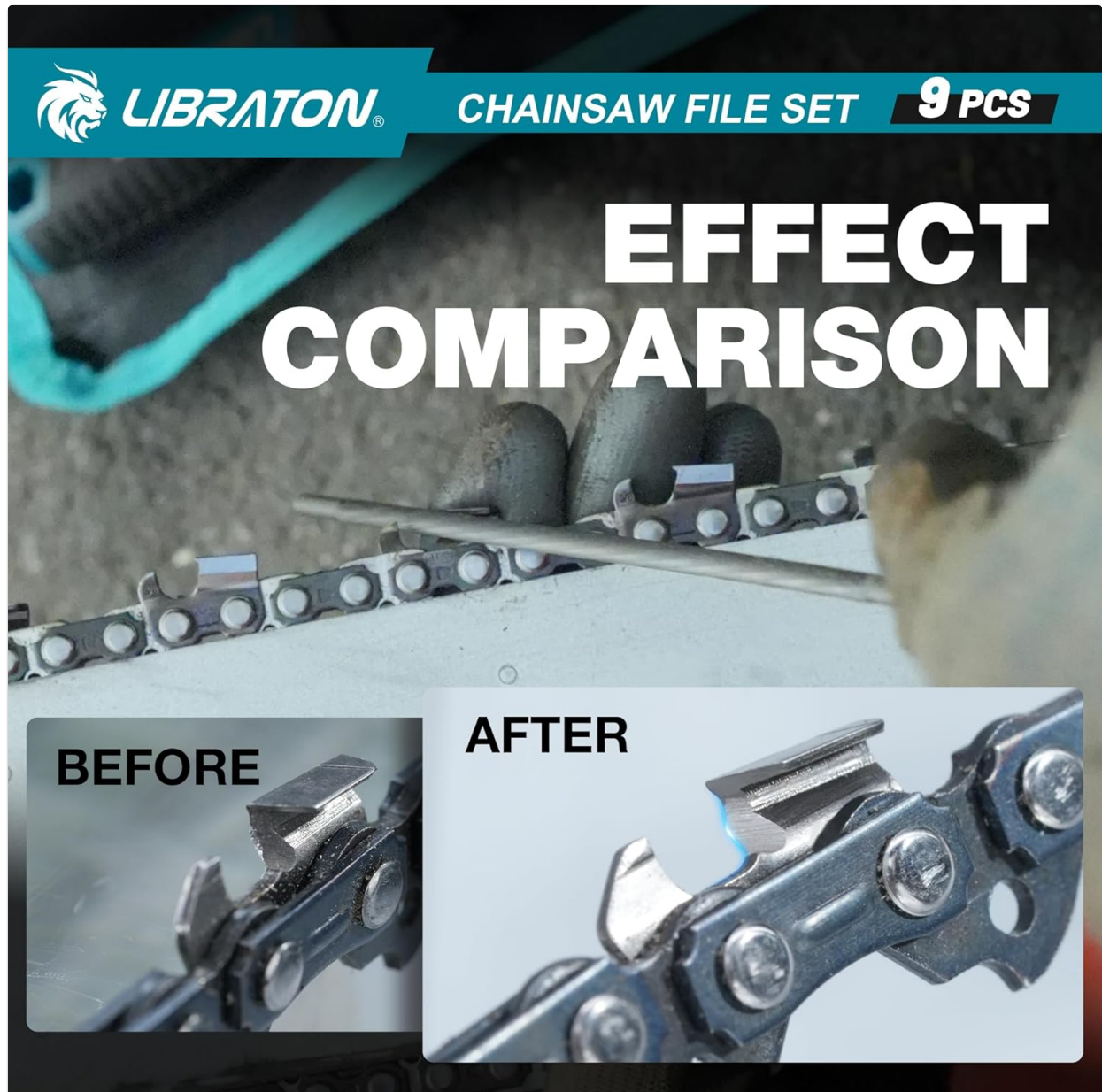
Figure 6: Visual comparison of a dull chainsaw tooth (left) and a properly sharpened tooth (right).
