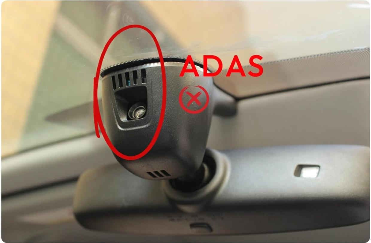
*Image: Warning against installation if an ADAS camera is present.*
