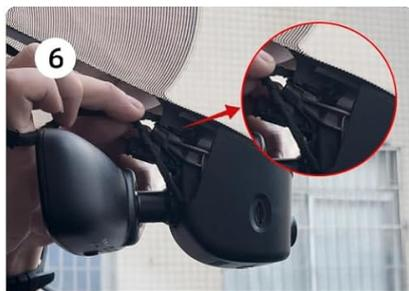
Connect the dash cam to the rain-fall sensor
