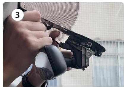
Take off the power supply of the rain-fall sensor
