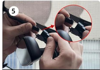
Connect the power supply to the dash cam
