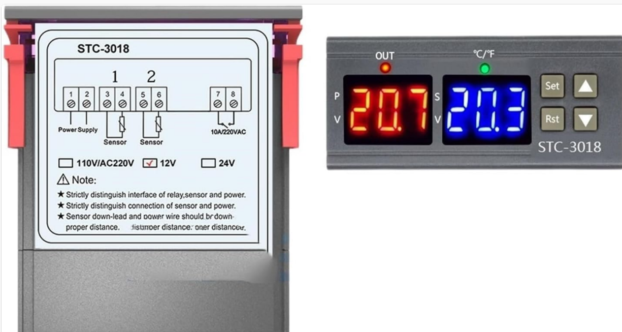
Figure 1: Wiring diagram for the STC-3018 controller. Terminals 1 and 2 are for power supply (DC 12V for this model). Terminals 3 and 4 are for the NTC temperature/humidity sensor. Terminals 5, 6, 7, and 8 are for the 10A/220VAC output relay connections.
