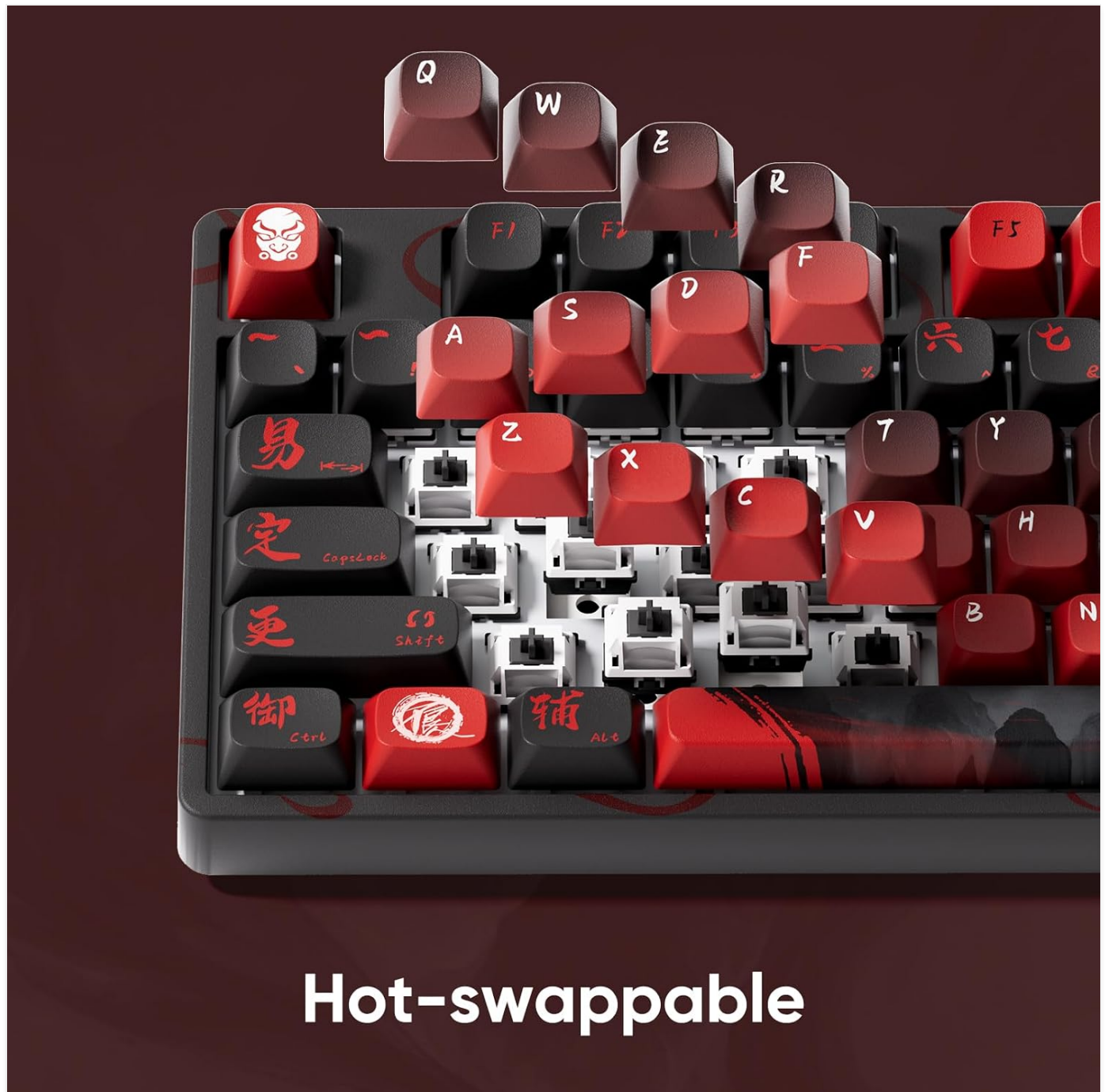
Figure 4: Hot-swappable sockets allowing for easy switch replacement.
