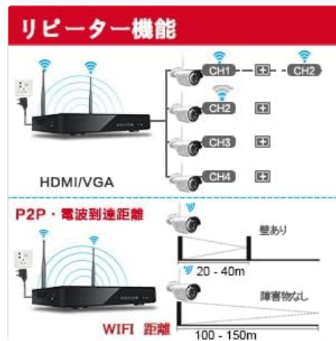
Figure 3.2: The top section shows the repeater function, where cameras can extend the signal range by relaying it through other cameras (CH1 to CH2, etc.). The bottom section illustrates the WiFi signal range: approximately 20-40 meters through wooden walls and 100-150 meters in an environment with a clear line of sight.
