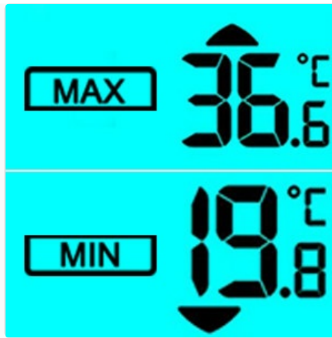
Image 4.3: Close-up of the display showing the recorded maximum (MAX) and minimum (MIN) temperature values.
