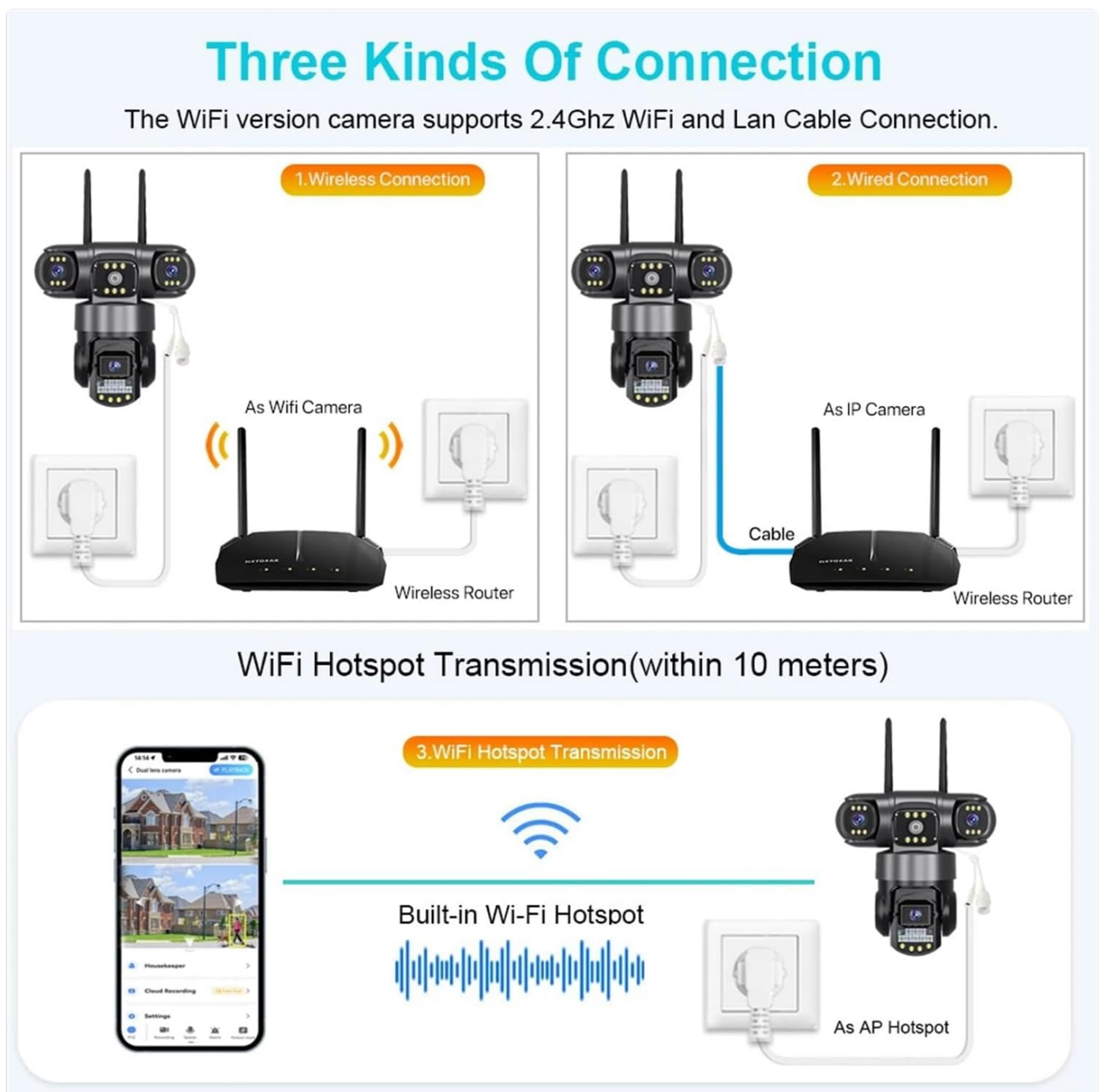
Figure 2: Various connection methods for the V380 Pro camera, including wireless via Wi-Fi, wired via Ethernet cable, and direct
