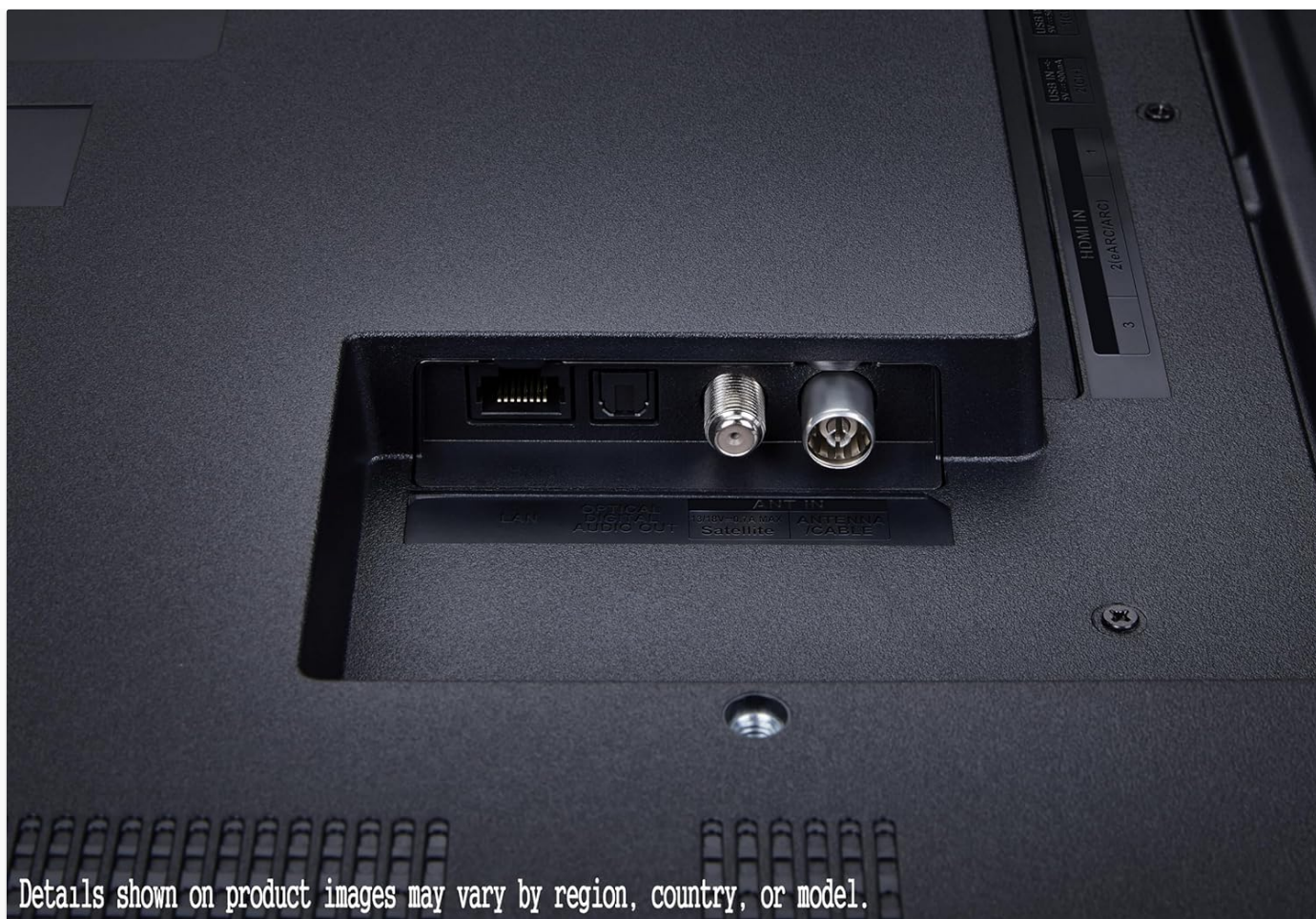
Rear view of the LG 50UA73 TV showing the LAN, Optical Audio Out, RF, and Satellite input ports.
