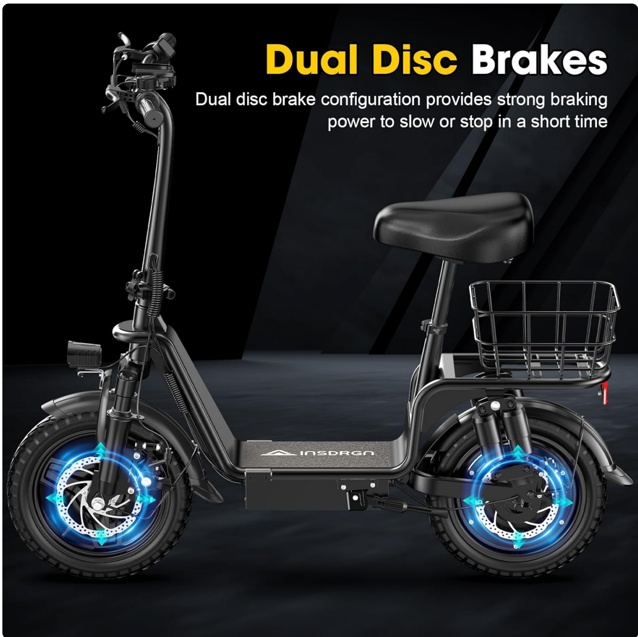
Figure 4.1: Dual disc brake system for strong braking performance.
