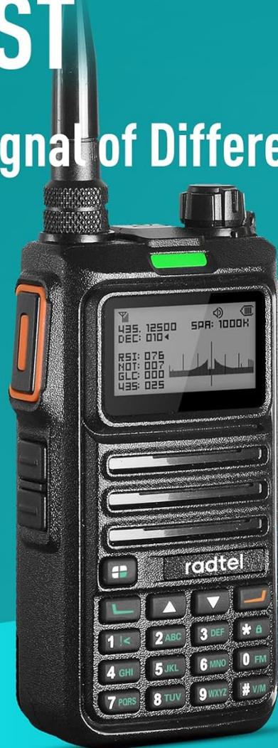
Figure 5: The Radtel RT-4D displaying its Spectrum Functions, including the TX Test for analyzing signals of different frequencies.
