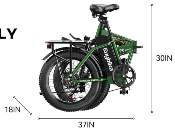
Figure 8.2: Diagram showing the dimensions, weight (63 lbs), maximum load capacity (330 lbs), and recommended rider height (5'3"-7'2") for the EUYBIKE F6.
