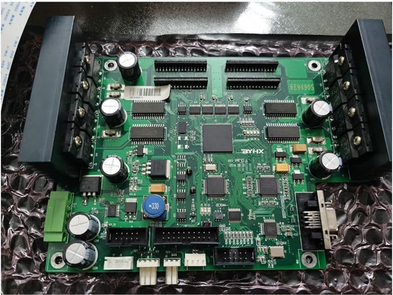
Figure 2.1: Overview of the BYHX DX5 Carriage Board. This image displays the main components and layout of the board, including integrated circuits, capacitors, and multiple connector ports for print heads and data cables.
