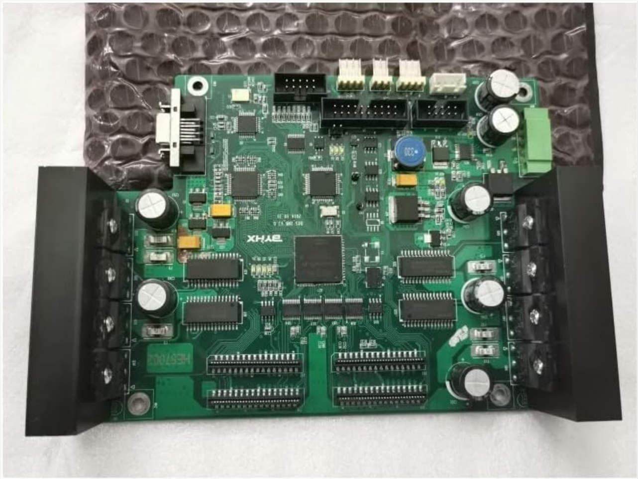
Figure 3.1: Top-down view of the BYHX DX5 Carriage Board. This image provides a clear view of all connection ports, which is essential for correct cable routing during installation.
