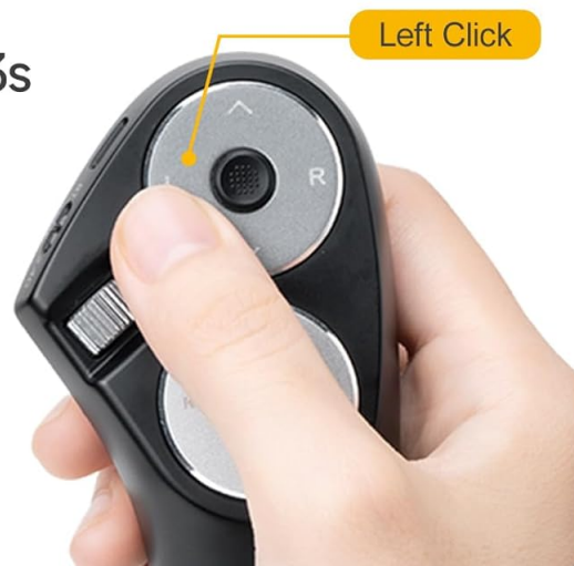
Image 3.2: Diagram illustrating the buttons for PowerPoint clicker functions, including Page Up/Down and Full/Black Screen.
