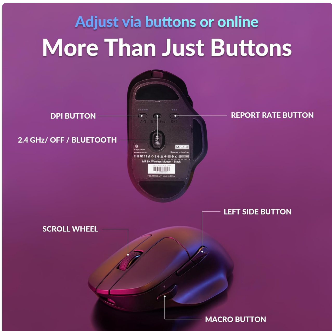
Image: An annotated diagram of the Keychron M7 8K Wireless Mouse, highlighting the DPI button, 2.4 GHz/OFF/Bluetooth switch, Report Rate button, Scroll Wheel, Left Side Button, and Macro Button.
