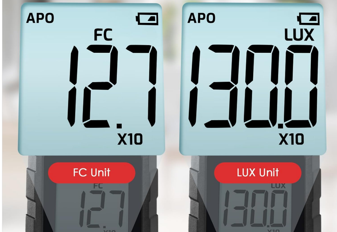
Figure 6.2: Explanation of how to interpret readings when 'X10' or 'X100' multipliers are active on the display.
