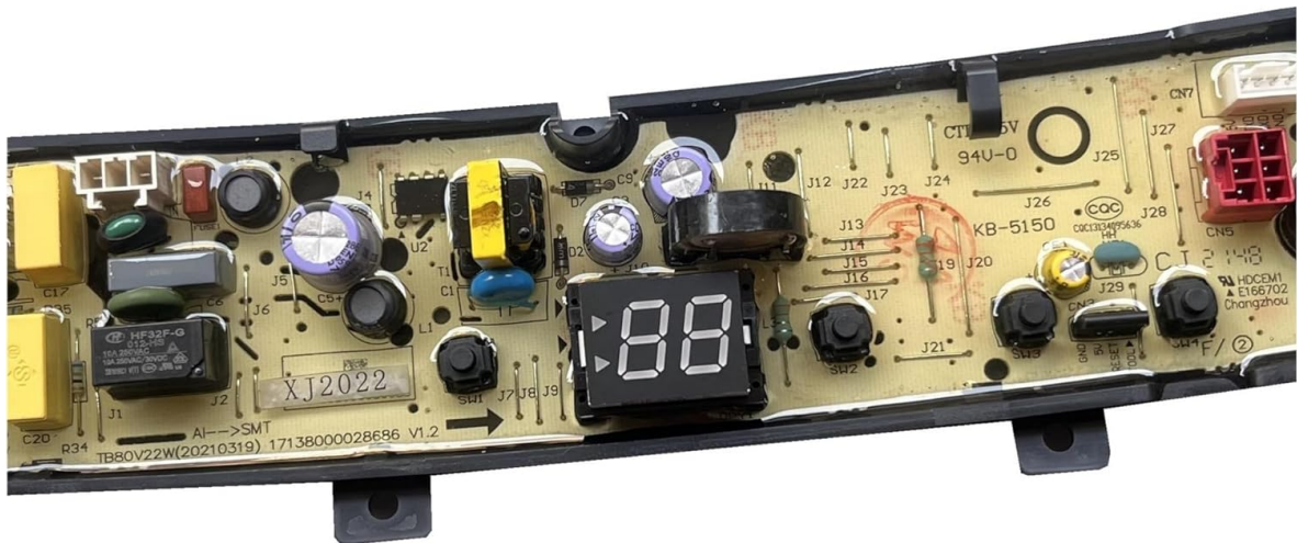
Figure 3.2: Detailed view of the XFHDHR Washing Machine Computer Board, focusing on the digital display and user interface elements. This perspective shows the '88' digital display, several push-buttons (SW1, SW2, SW3), and various surface-mounted components. The board's model number "TB80V22W" and revision "V1.2" are also visible.
