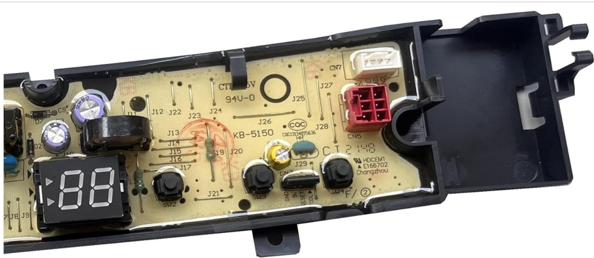
Figure 3.3: Side view of the XFHDHR Washing Machine Computer Board, emphasizing the main connectors. This image provides a clearer view of the multi-pin connectors (CN5, CN7) and the power input section. The overall robust construction of the board and its protective casing are also evident.
