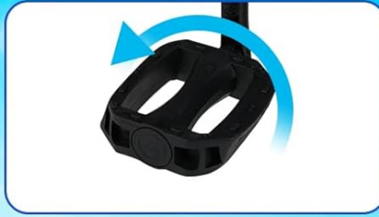
Coaster Brake Pedal backwards to stop
