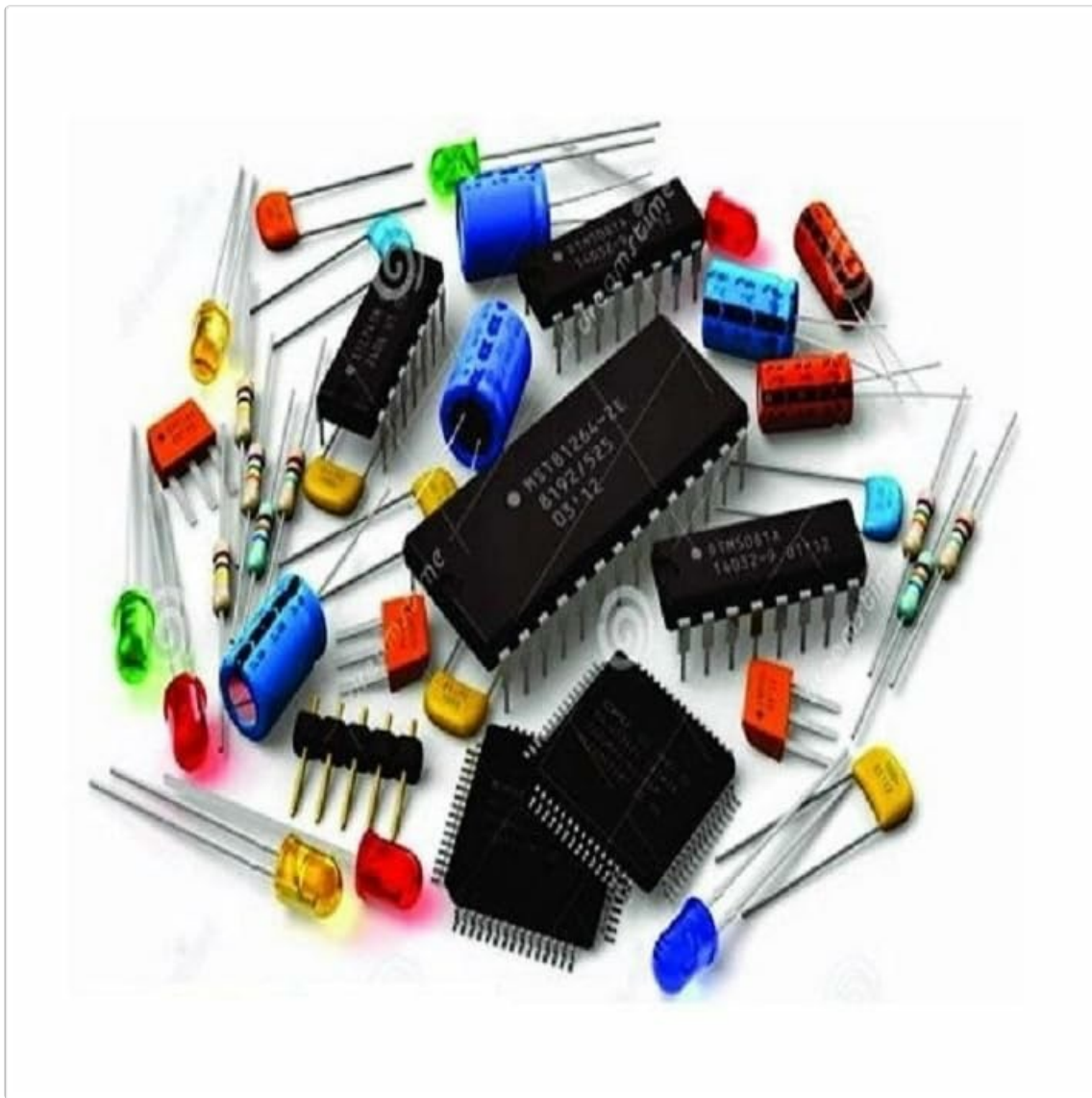
Image: Various electronic components, including integrated circuits, resistors, capacitors, and LEDs, are shown, representing the parts included in the kit for assembly.
