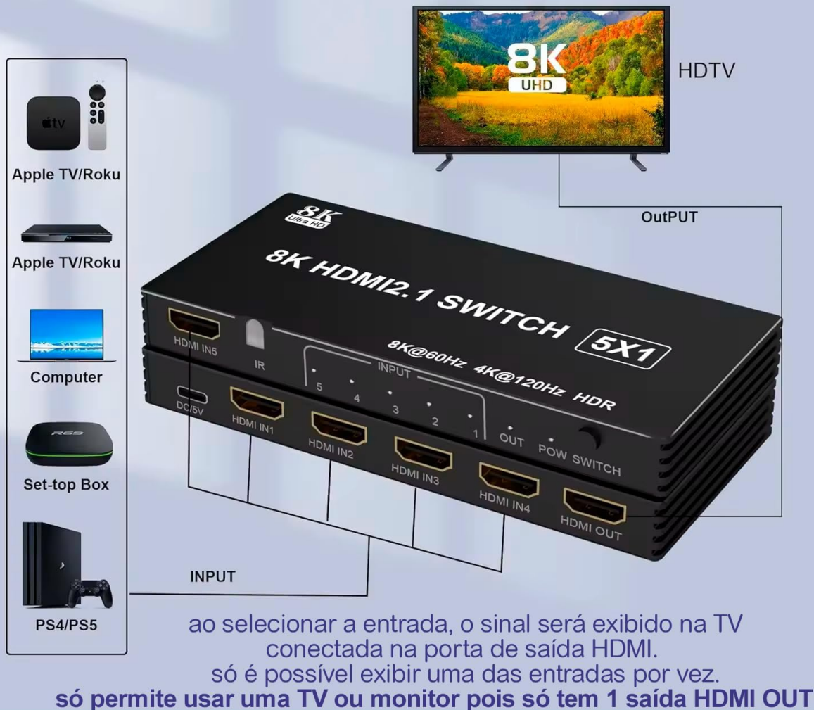
Image 5.1: Connection diagram illustrating how to link multiple HDMI sources to the switch and a single display.
