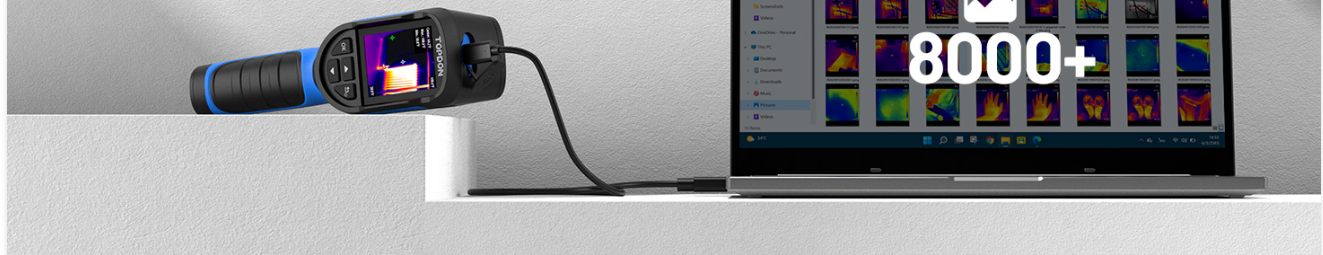
Figure 5.4: The TC004 Mini connected to a laptop, illustrating the process of exporting stored thermal images.
