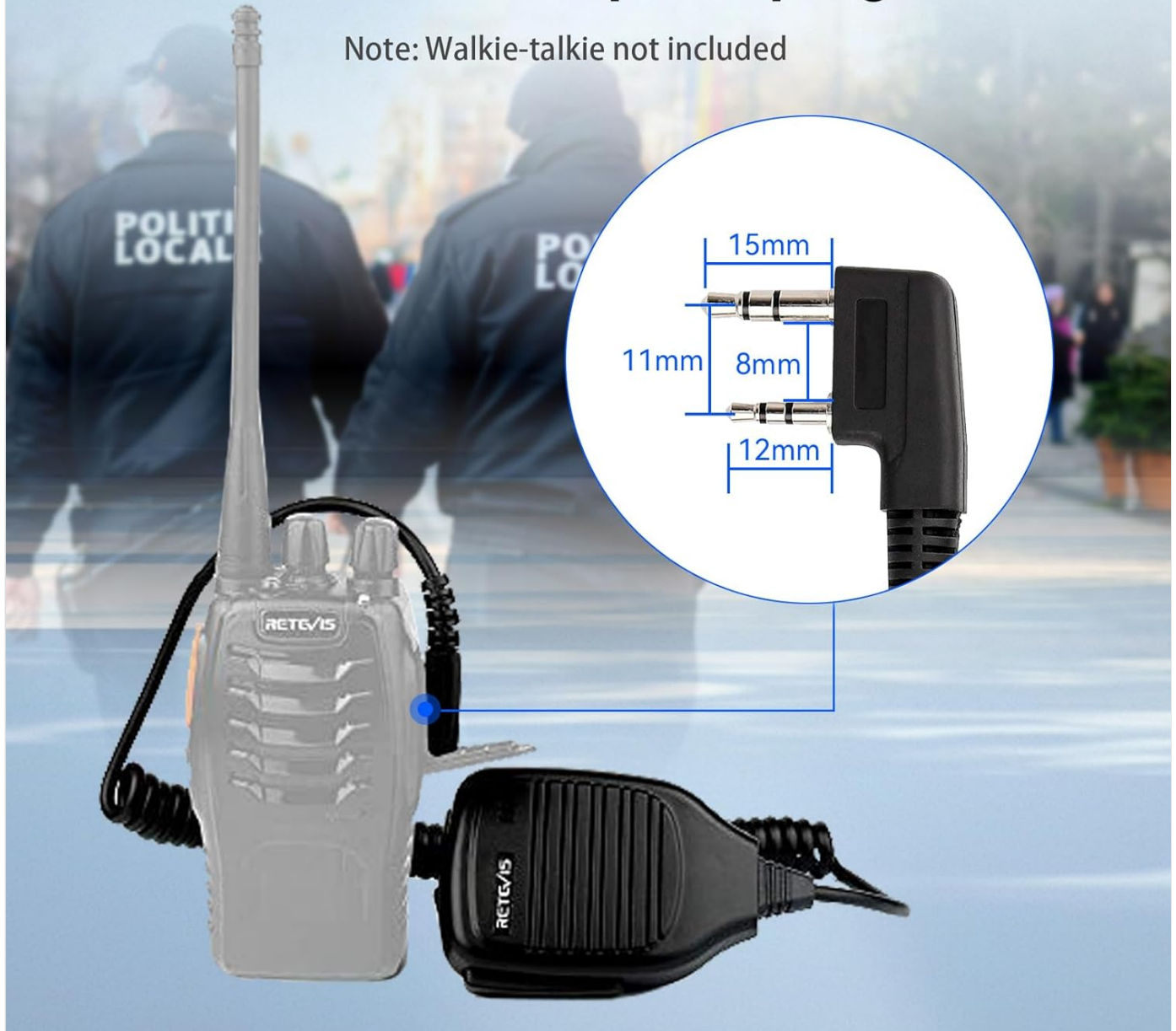
Figure 2.6: Illustration showing the standard 2-pin K plug dimensions and its connection to a walkie talkie.
