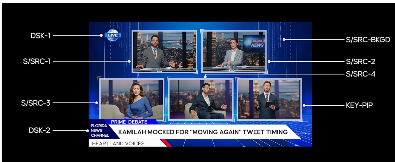
Figure 10: The 8-layer composition engine for complex visual arrangements.
