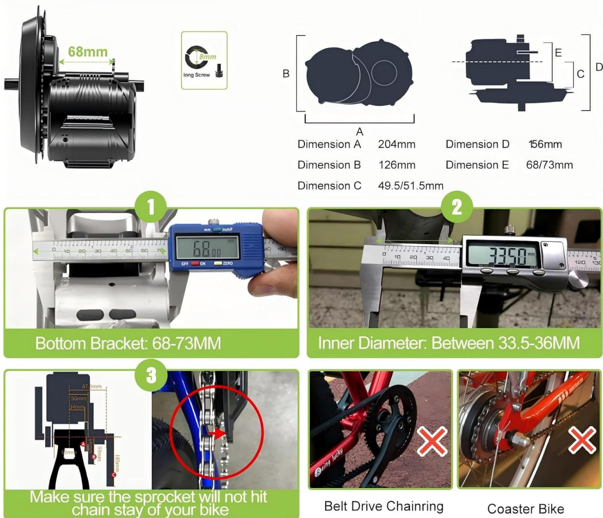
Image 4.1: Instructions for measuring your bike's bottom bracket to ensure compatibility with the mid-drive motor. It also shows examples of incompatible chainring and coaster brake setups.
