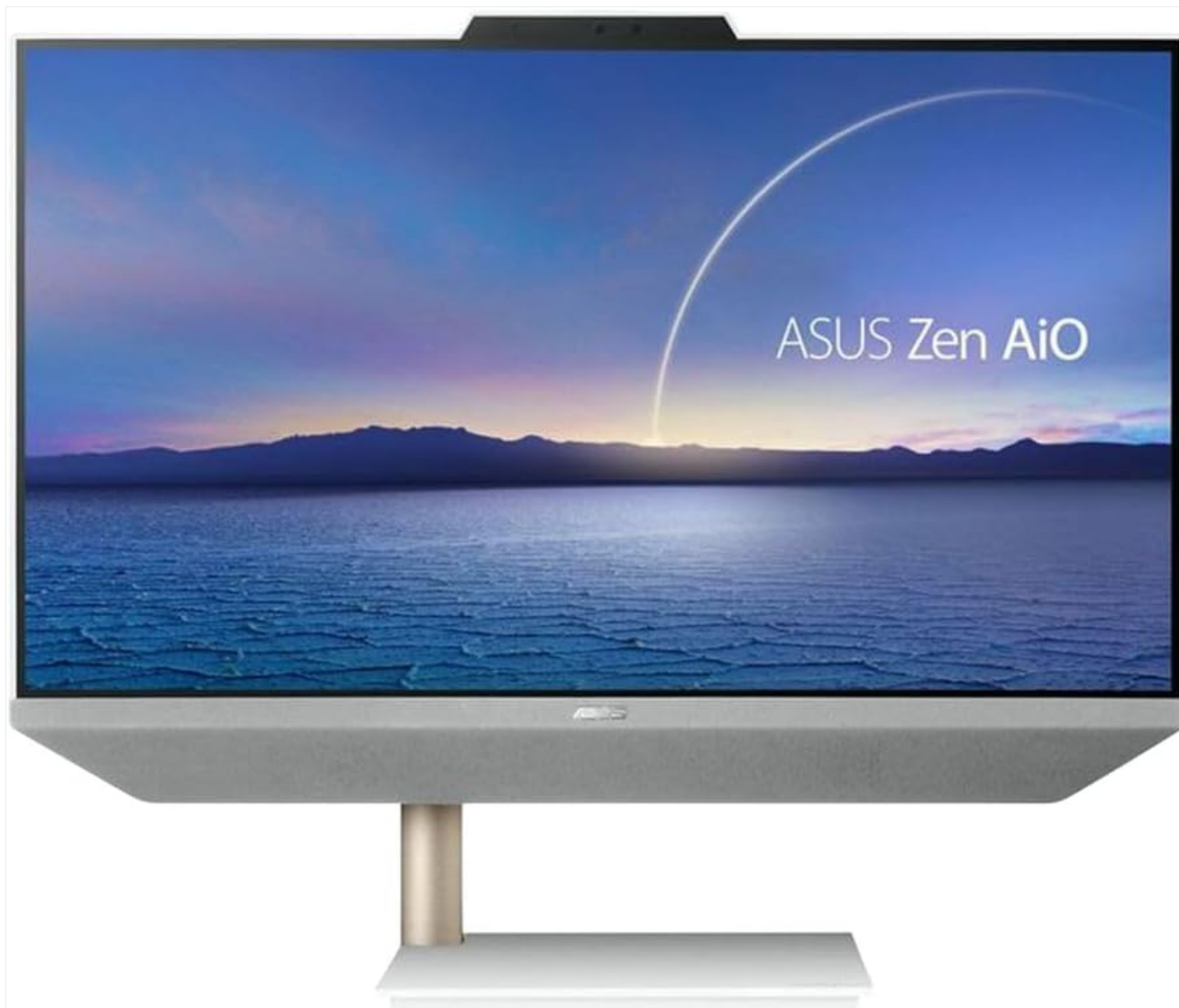
Figure 2.1: Front View. The ASUS Zen AiO features a 23.8-inch Full HD touchscreen display with a narrow bezel, and a speaker bar integrated below the screen. The webcam is located at the top center of the display.
