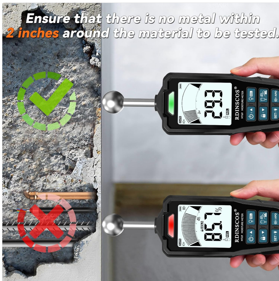
Figure 8: Illustration showing correct measurement without metal interference and incorrect measurement with metal interference.
