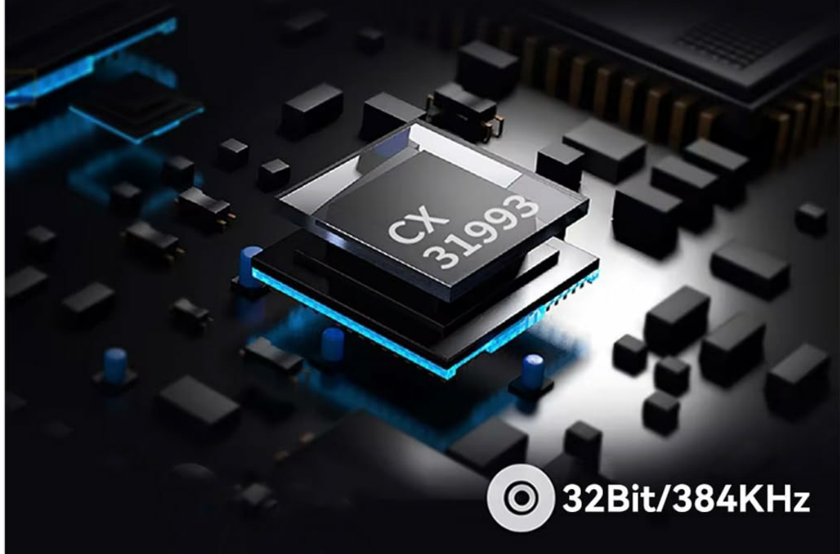
Image 7.1: A detailed view of the Conexant CX31993 digital audio decoder chip, highlighting its role in delivering 32-bit/384kHz audio resolution.
