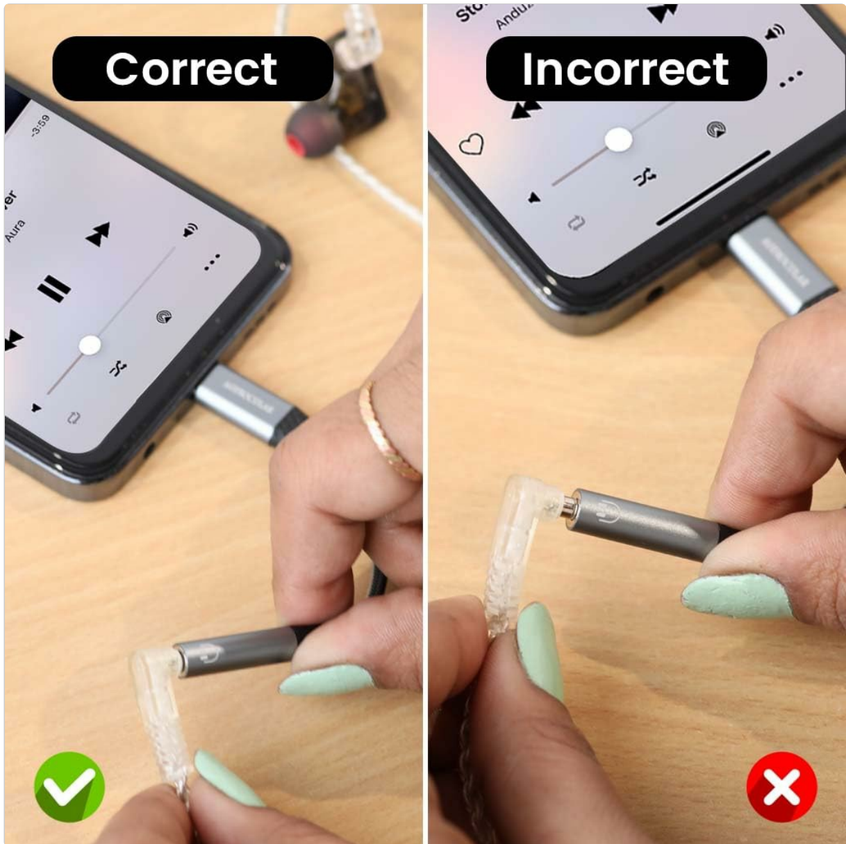
Image 4.4: Visual guide demonstrating the correct and incorrect methods for connecting a 3.5mm audio jack to the dongle, ensuring a secure and functional connection.
