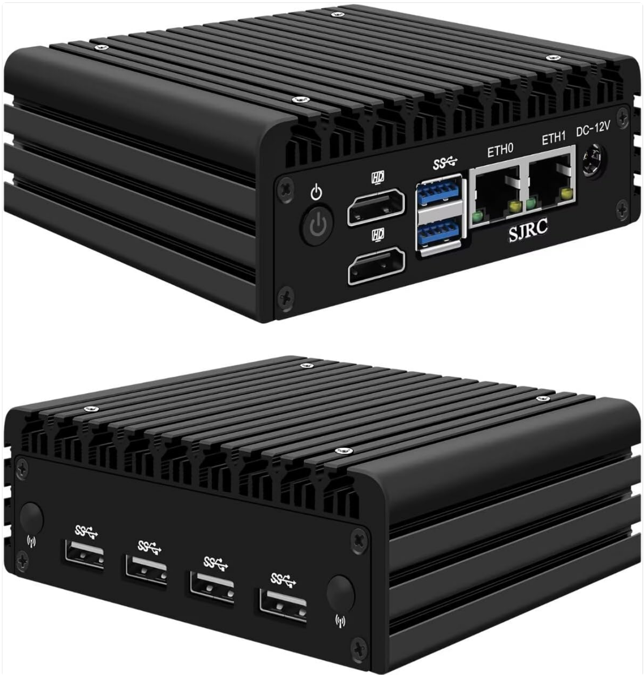
Figure 4.1: Front and rear views of the SJRC X86 P6 Mini PC. The front panel includes the power button, two HD ports, and two USB 3.2 ports. The rear panel features two 2.5GbE LAN ports (ETH0, ETH1) and the DC-12V power input.
