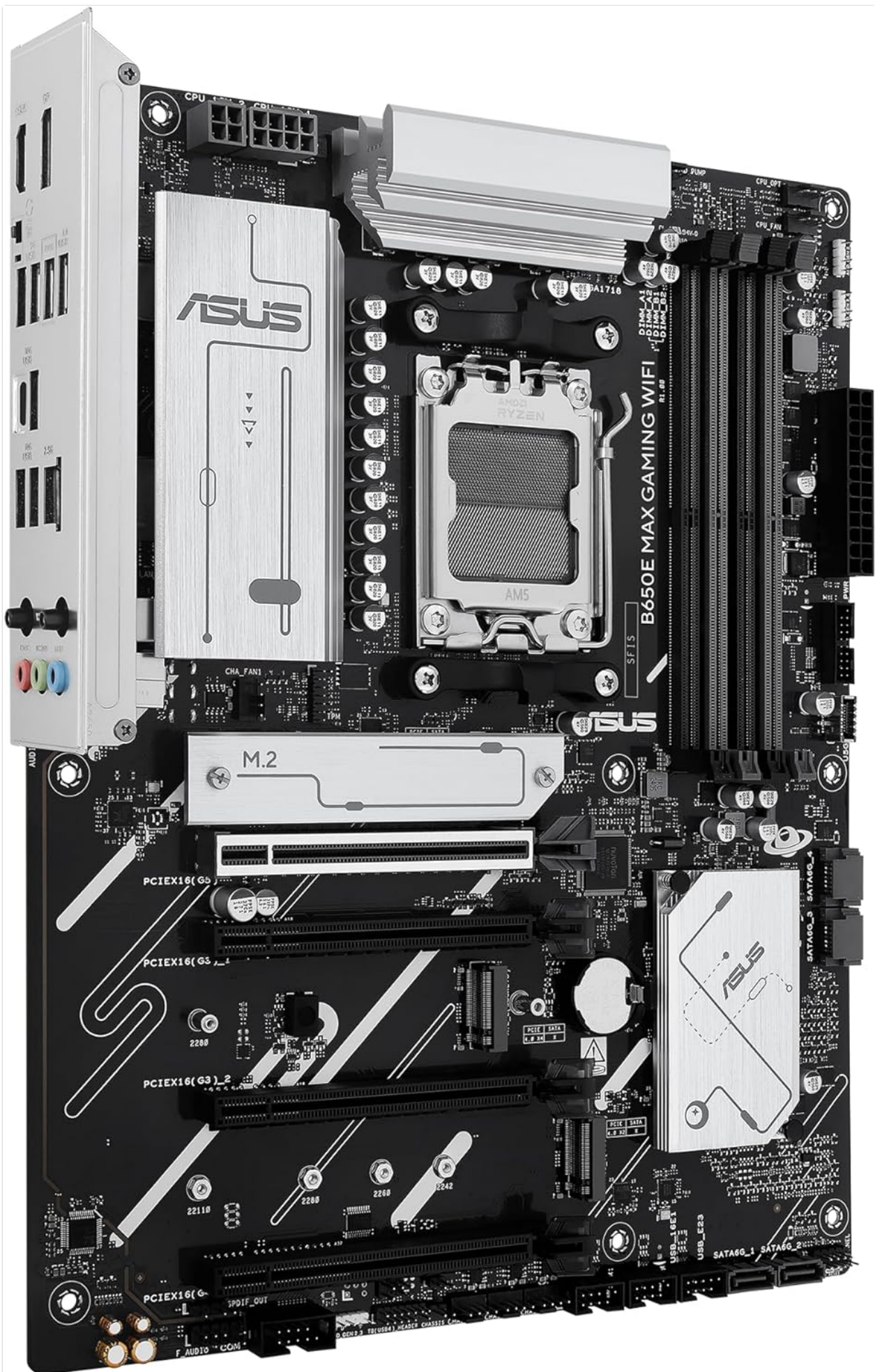
Image: A top-down view of the ASUS B650E MAX Gaming WiFi Motherboard, highlighting the CPU socket, DDR5 DIMM slots, PCIe slots, and M.2 slots.
