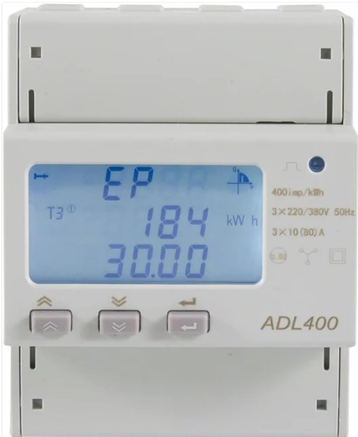
Image 5.1: ADL400 Display. This image shows the ADL400 energy meter's LCD display, indicating 'EP' (Energy Positive) and a reading of '184 kWh' for total active energy. Below that, '30.00' is displayed, which could represent instantaneous power or another parameter. The display also shows '400 imp/kWh', '3x220/380V 50Hz', and '3x10(80)A', indicating the meter's pulse constant, voltage rating, frequency, and current rating.
