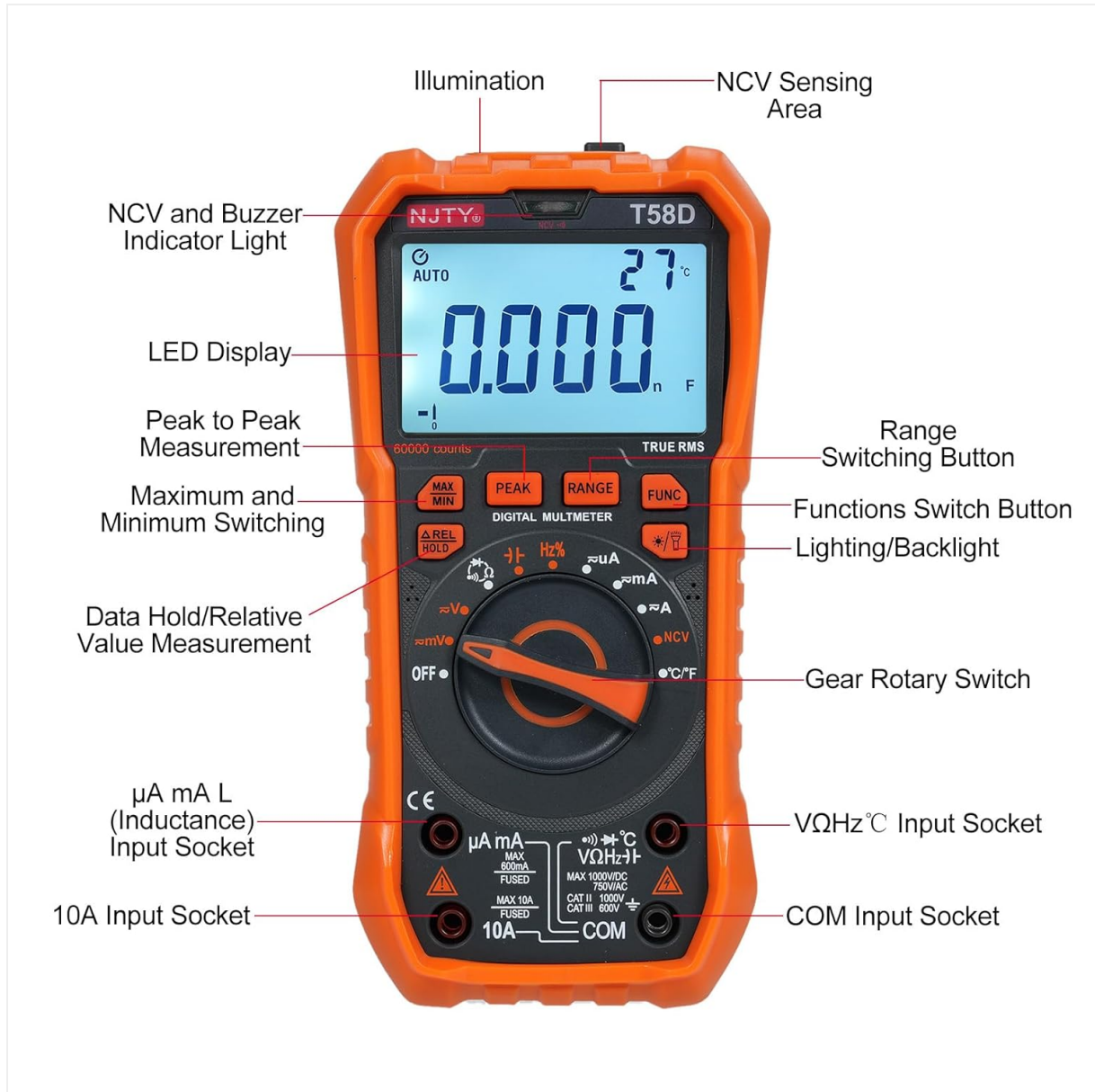
Figure 4.1: Front view of the NJty T58D Digital Multimeter with key components labeled. Labels include LED Display, NCV Sensing Area, Illumination, NCV and Buzzer Indicator Light, Peak to Peak Measurement, Maximum and Minimum Switching, Data Hold/Relative Value Measurement, Range Switching Button, Functions Switch Button, Lighting/Backlight, Gear Rotary Switch, \mu\text{A} mA L (Inductance) Input Socket, 10A Input Socket, V \Omega Hz ^{\circ}\text{C} Input Socket, and COM Input Socket.
