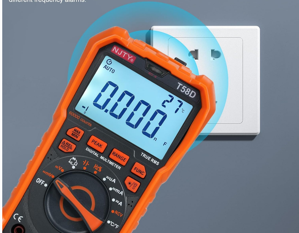
Figure 6.2: Demonstrates the NCV function, where the top of the multimeter is placed near an AC voltage source to detect its presence without direct contact. The device indicates voltage intensity through visual and audible alerts.
