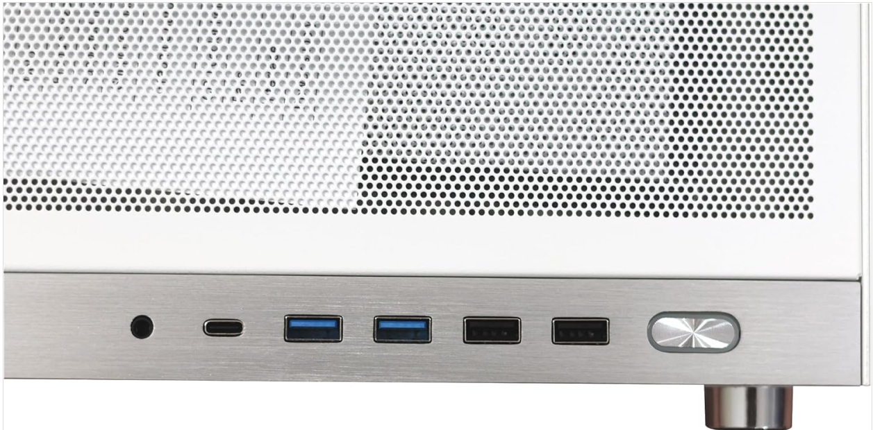
Figure 10: Close-up of the front I/O ports, including USB 3.0, USB 2.0, Type-C, and audio jack.
