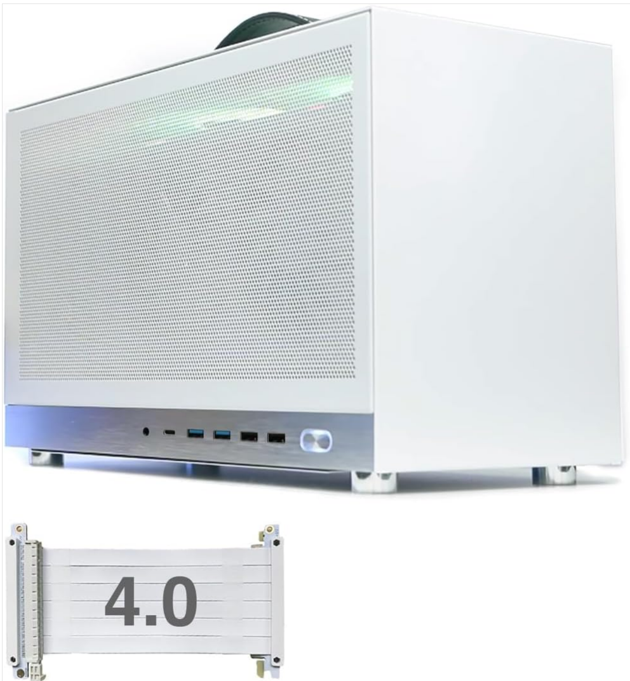
Figure 1: MININGEEK S400 Pro Mini-ITX Computer Case with included PCIe 4.0 riser cable.
