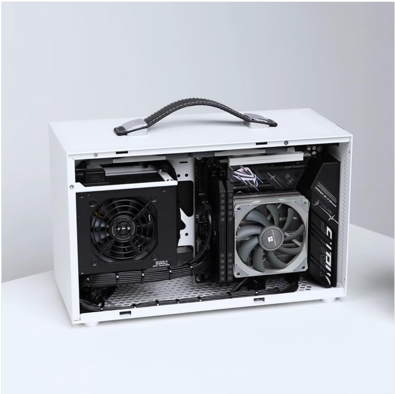
Figure 2: Case dimensions (Length: 340mm, Width: 155mm, Height: 205mm).
