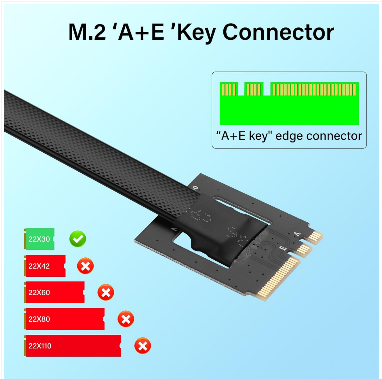
Figure 1: M.2 Key A+E Connector. This image shows the M.2 'A+E' Key Connector end of the extender cable, highlighting its compatibility with 2230 size M.2 slots.
