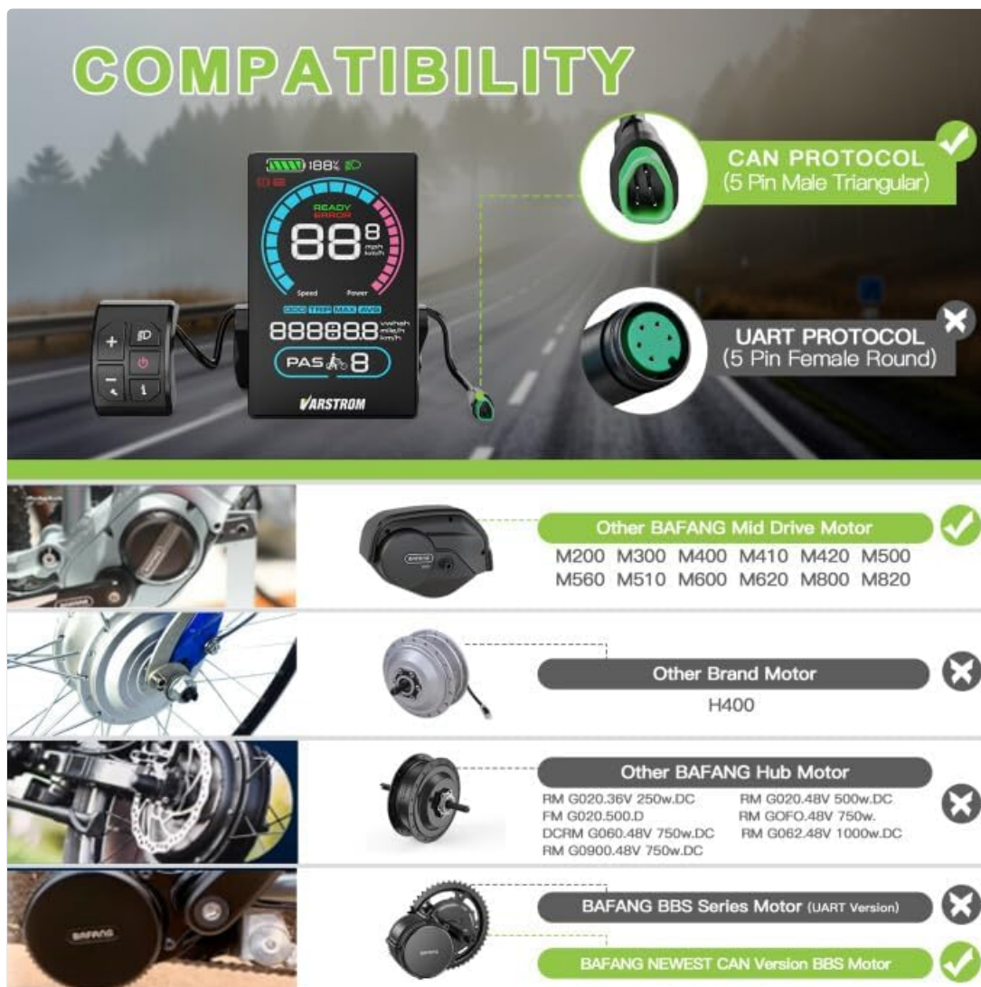
Figure 2.1: VD618 Compatibility Overview. This diagram illustrates the correct CAN protocol connector (5-pin male triangular) required for the VD618 display and lists compatible Bafang mid-drive motors (M200, M300, M400, M410, M420, M500, M560, M510, M600, M620, M800, M820 CAN Version) while indicating incompatibility with UART protocol motors and certain hub motors.
