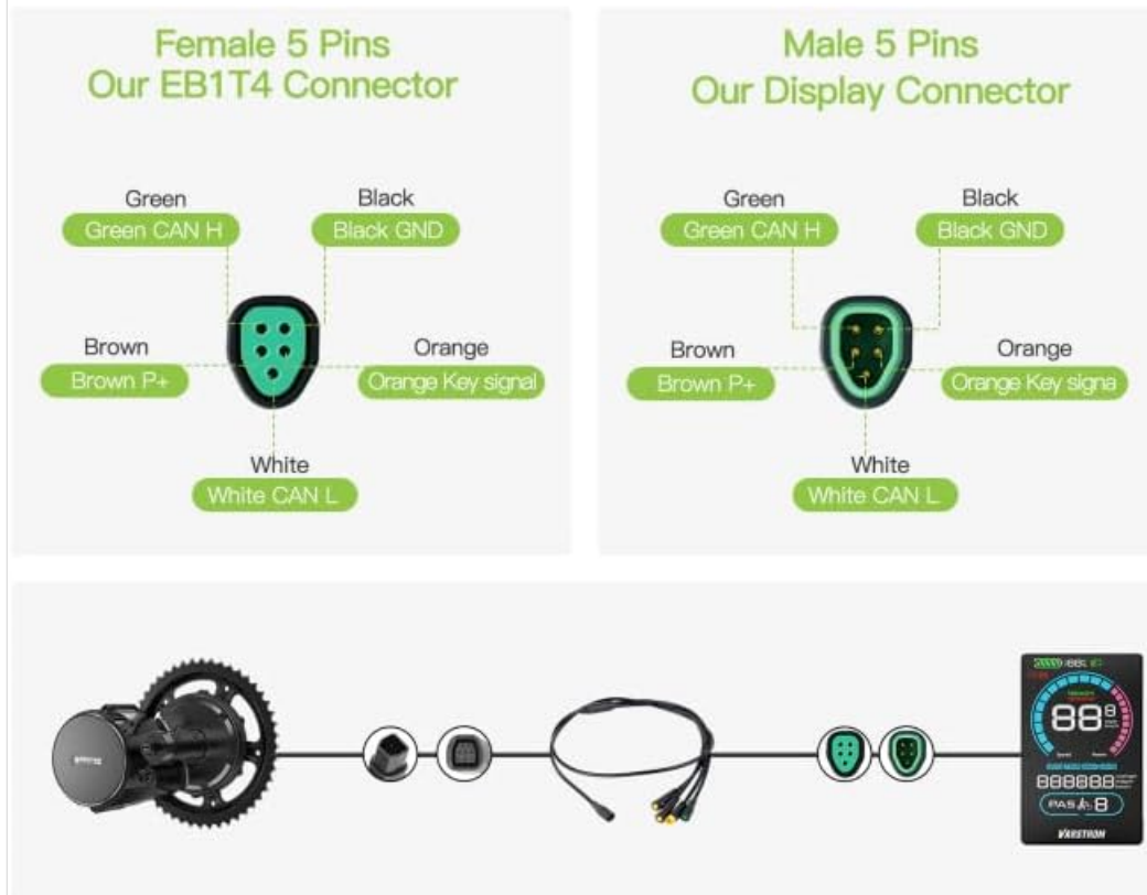
Figure 3.2: Cable Parameters and Wiring Diagram. This diagram details the wiring connections between the e-bike's 1T4 cable and the VD618 display, showing the function of each of the five pins (Green CAN H, Black GND, Brown P+, Orange Key signal, White CAN L).
