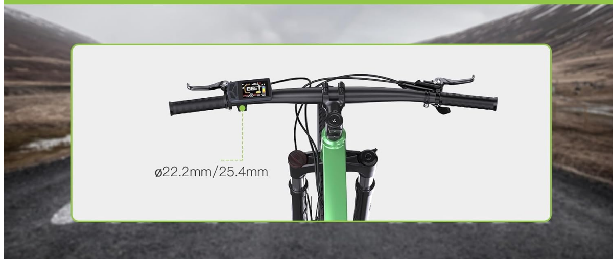
Figure 3.2: Illustration of handlebar compatibility, showing the display's adjustable mount for 22.2mm and 25.4mm handlebars.
