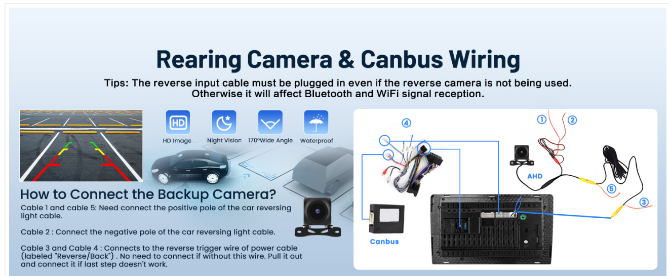
Figure 3: Wiring connections for the radio and reverse camera.
