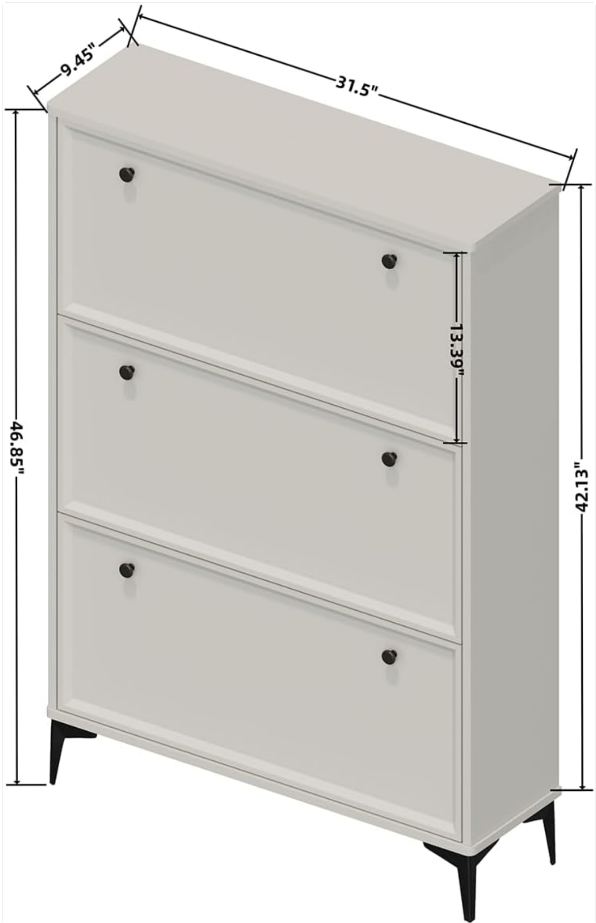
Image 8.1: Dimensional drawing of the shoe cabinet, indicating its height, width, and depth.
