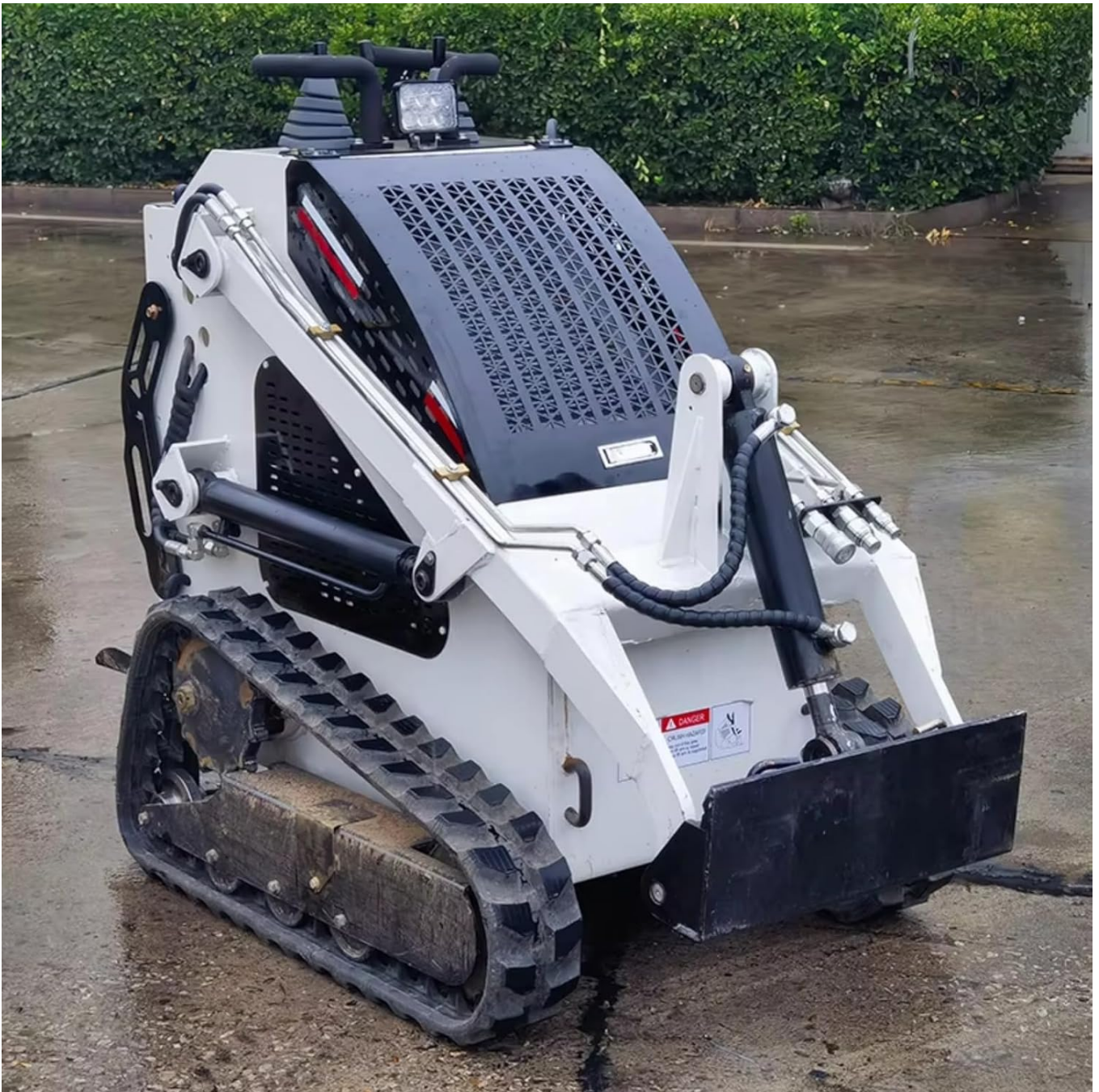
Image: White tracked skid steer loader, demonstrating another color option and the tracked design.
