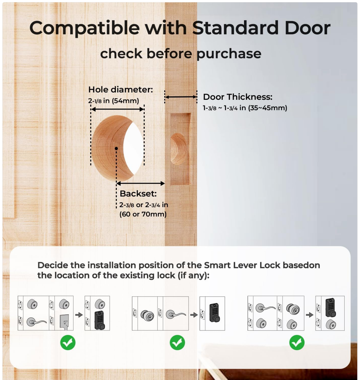
Figure 1: Door compatibility dimensions for installation.
