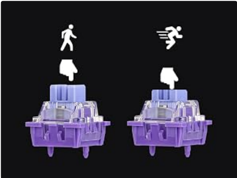
Image: An illustration of the Dynamic Key Stroke (DKS) functionality, where pressing a key to different depths can activate distinct commands, such as walking or running in a game.
