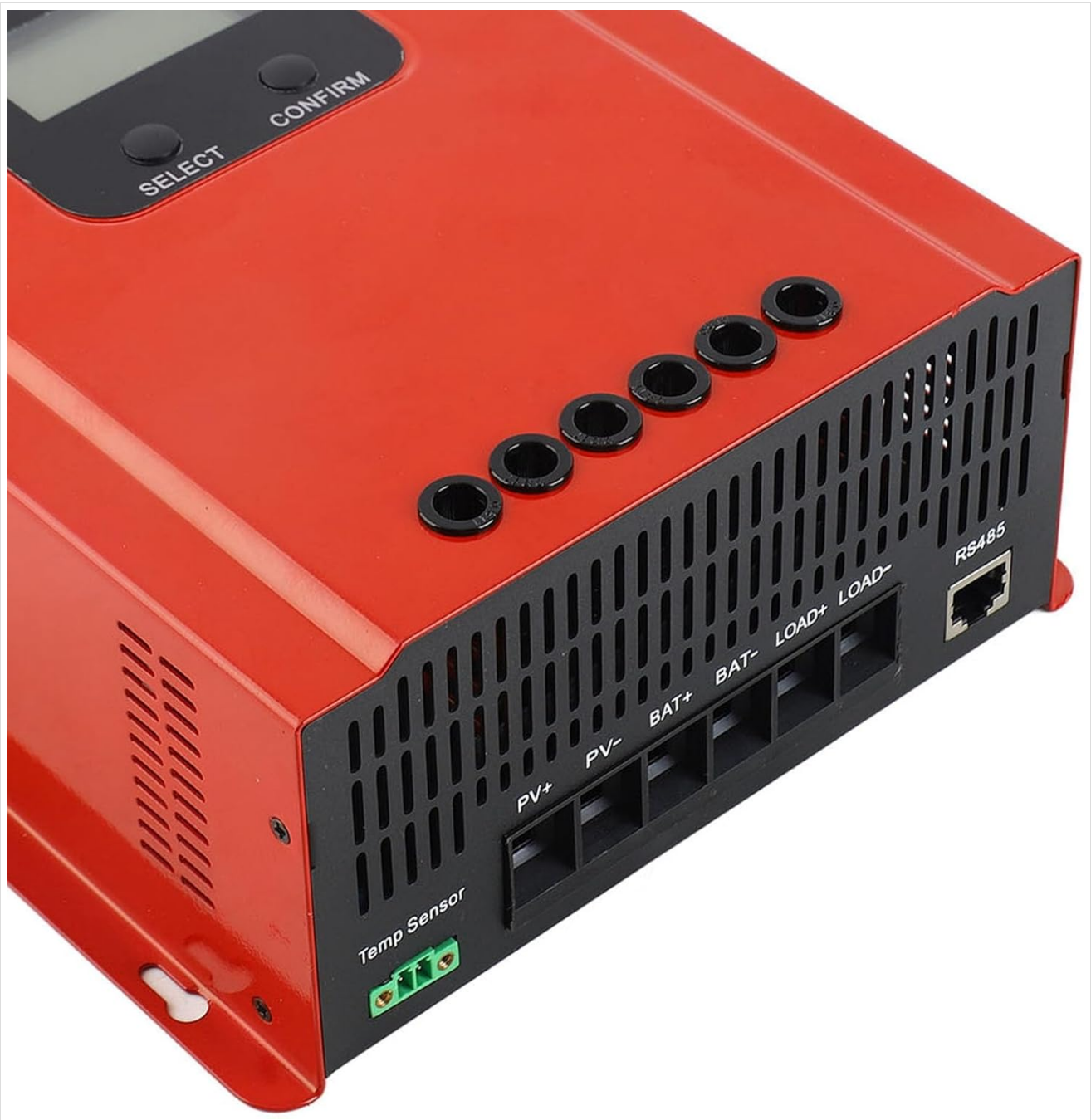
Figure 2: Connection Terminals. This image highlights the various input and output terminals on the controller for solar panels, battery, load, temperature sensor, and RS485 communication.
