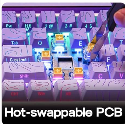
Image 5.5: The hot-swappable design allows for easy switch replacement.
