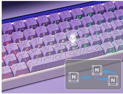
Image 5.1: Visual representation of adjustable actuation for magnetic switches.
